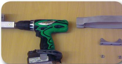
*Lock arm that disables torsion. A lock arm that's mounted on the drill and the Net-tester 200H can be provided. This provides the Net-tester 200H from torsion during tests of the netting yarn.*
