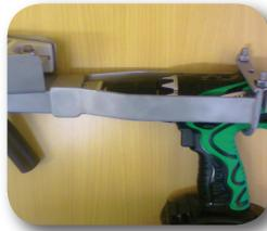
Place the hoop and tighten both nuts (13mm nut key) until it is properly fasten to the drill.
