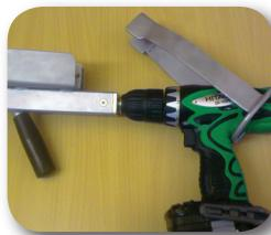
Lead the lock arm over the drill and place it on the Net-tester 200H.
